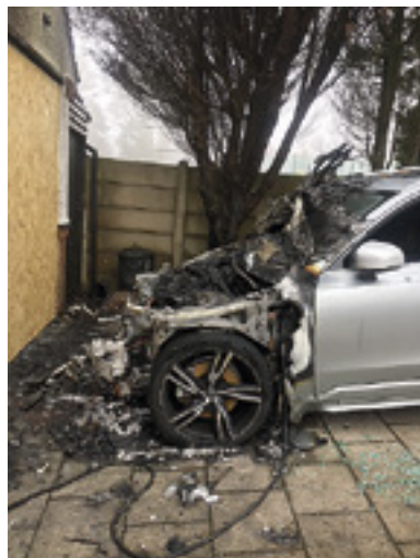
Fig 2: Colleague's Volvo hybrid EV caught fire overnight whilst on charge
