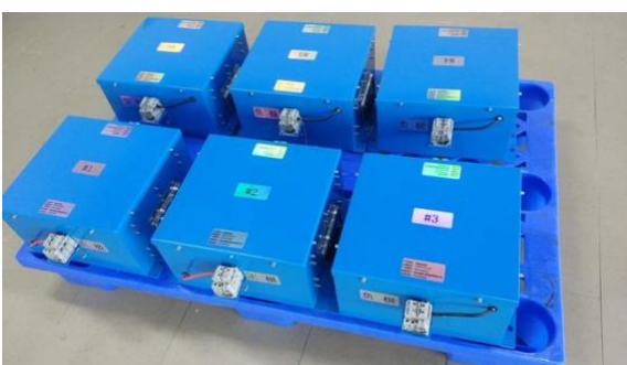
Figure 2: The six power capacitor modules used for the pitch backup power supply.
