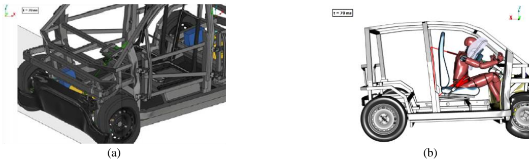
Fig. 2. (a) Simulation results of the Multi-Moby vehicle under the R137 crash, after structure optimisation; and (b) analysis of the restraint system under the R137 crash.
